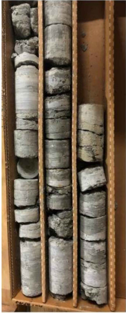
Rock core from boring B-038-0-20, 28.8 to 33.8 ft.
