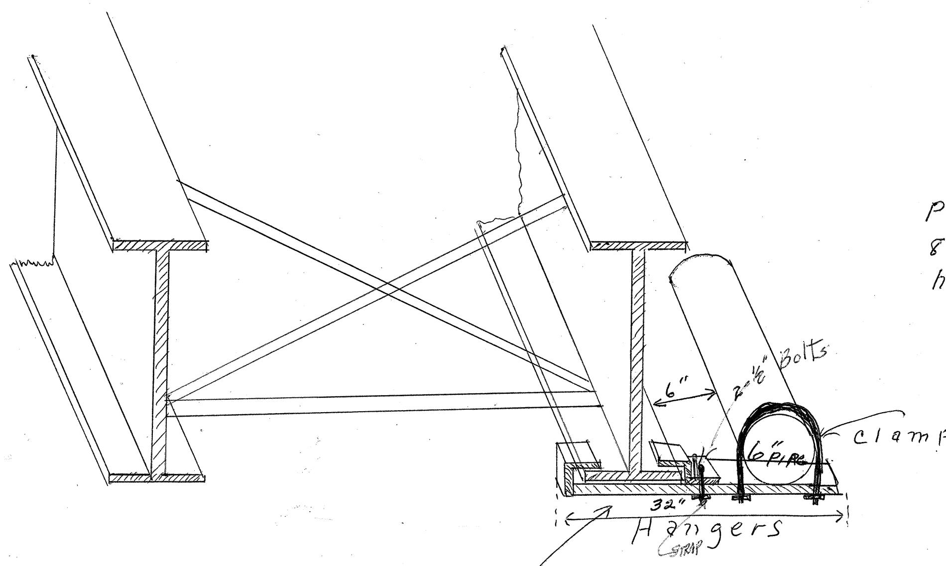
Brackets of 1" iron to be used on bridge deck
