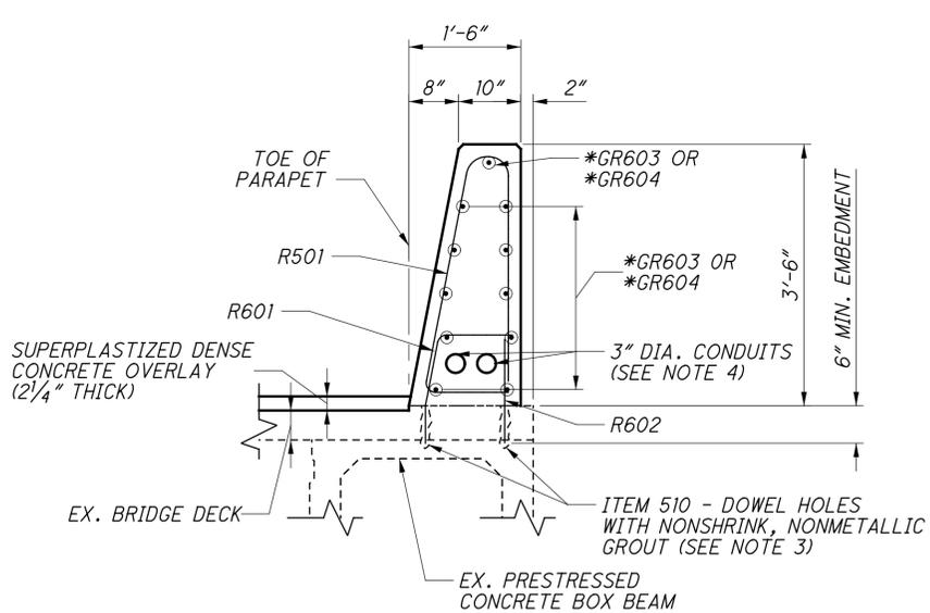
**TYPICAL PARAPET SECTION**
