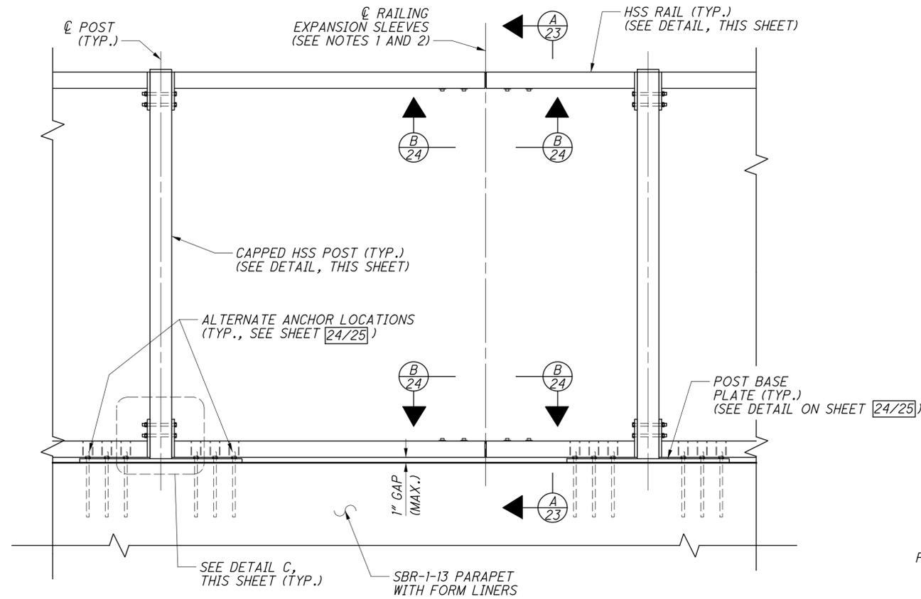
**TYPICAL STRUCTURAL FRAMING - INTERIOR ELEVATION**
