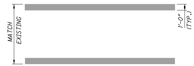
FINAL CROSSWALK MARKING DETAIL (LONGITUDINAL LINES ONLY)
