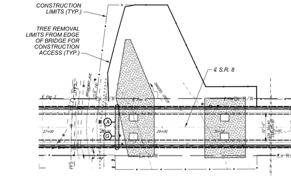
CONSTRUCTION LIMITS AT PIERS 4 & 5 DETAIL
