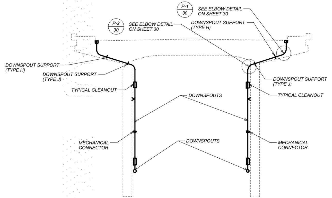
TYPICAL COLUMN DRAINAGE - ARCH SPANS
