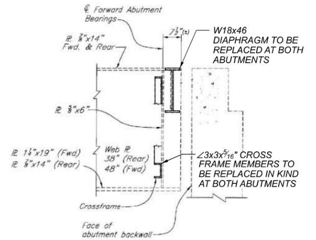
**FRAMING DETAIL AT ABUTMENTS**
