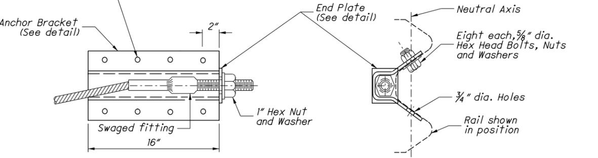
**ANCHOR BRACKET ASSEMBLY DETAILS**
