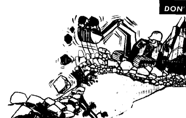
DON'T EPM No. 31.—Excavation of blasted material shall be conducted in such a manner that operation of excavation equipment does not contribute to loss of material down the slope. (See DO for proper procedure.)
