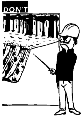
DON'T EPM No. 31.—In other than solid rock, the tops of excavated slopes shall be rounded off as shown on the contract drawings.
