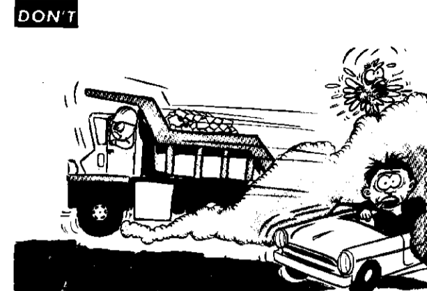
DON'T EPM No. 22.—The Contractor shall maintain all excavations, embankments, stockpiles, roads, plant sites, waste areas, borrow areas, and all other work areas within or without the project boundaries free from dust which would cause a hazard or nuisance to others.
