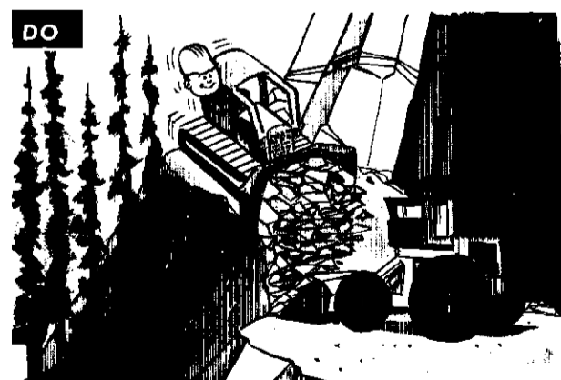
DO EPM No. 30.—Full U-blades shall be used on dozers excavating on slopes.
