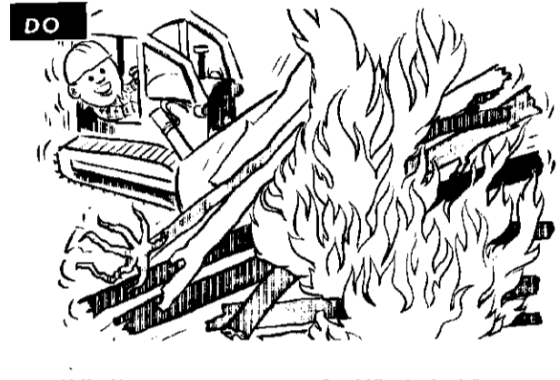
DO EPM No. 24.—Except as restricted by the Fire Control Officer, burning shall assure continuous, rapid and complete combustion. To meet this requirement, burning piles shall be kept under constant attendance by heavy equipment and operators who shall stack or push in burning piles from the edges, or shall feed fire with additional combustibles.
