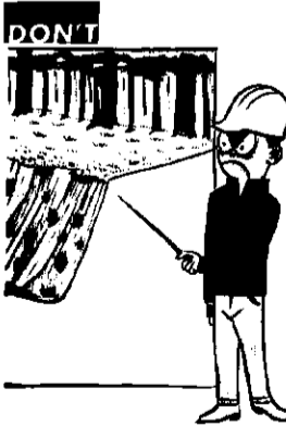
DON'T EPM No. 31.—In other than solid rock, the tops of excavated slopes shall be rounded off as shown on the contract drawings.
