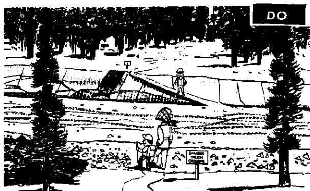
EPM No. 11. —Ramps shall be constructed in cut areas or trails shall be resealed to provide access. Location of rerouted trails shall be subject to the approval of the Contracting Officer. Traffic warning signs shall be provided at hiking trails and maintained during construction operations.
