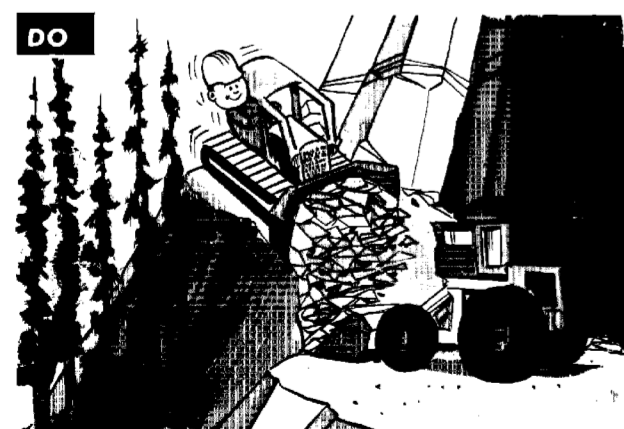
EPM No. 30. —Full U-blades shall be used on dozers excavating on slopes.
