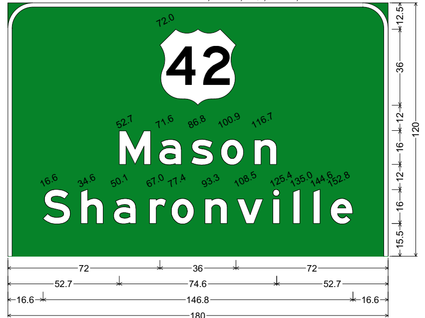
12.0" Radius, 2.0" Border, White on Green; US 42 M1-4; "Mason", E Mod 2K; "Sharonville", E Mod 2K;
