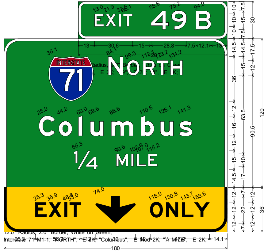
12.0" Radius, 2.0" Border, Black on Yellow; "EXIT", E 2K; Down Arrow C-1 - 22.0" 270"; "ONLY", E 2K;
