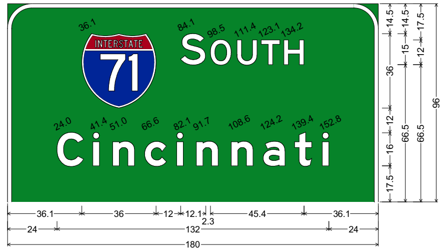
12.0" Radius, 2.0" Border, White on Green; Interstate 71 M1-1; "SOUTH", E 2K; "Cincinnati", E Mod 2K;
