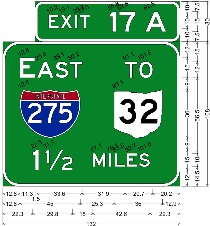
12.0" Radius, 2.0" Border, White on Green; "EAST", E 2K; "TO", E 2K; Interstate 275 M1-1; State Highway 32 M1-H5-36-2; "1 1/2 MILES", E 2K;
