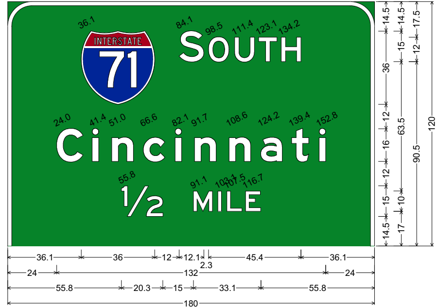
12.0" Radius, 2.0" Border, White on Green; Interstate 71 M1-1; "SOUTH", E 2K; "Cincinnati", E Mod 2K; "1/2", E 2K; "MILE", E 2K; "", E 2K;
