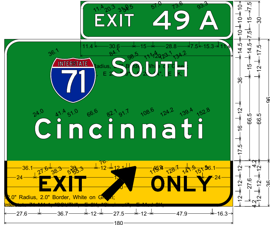
12.0" Radius, 2.0" Border, Black on Yellow; "EXIT", E 2K; Arrow A-1 - 35.0" 45°; "ONLY", E 2K;
