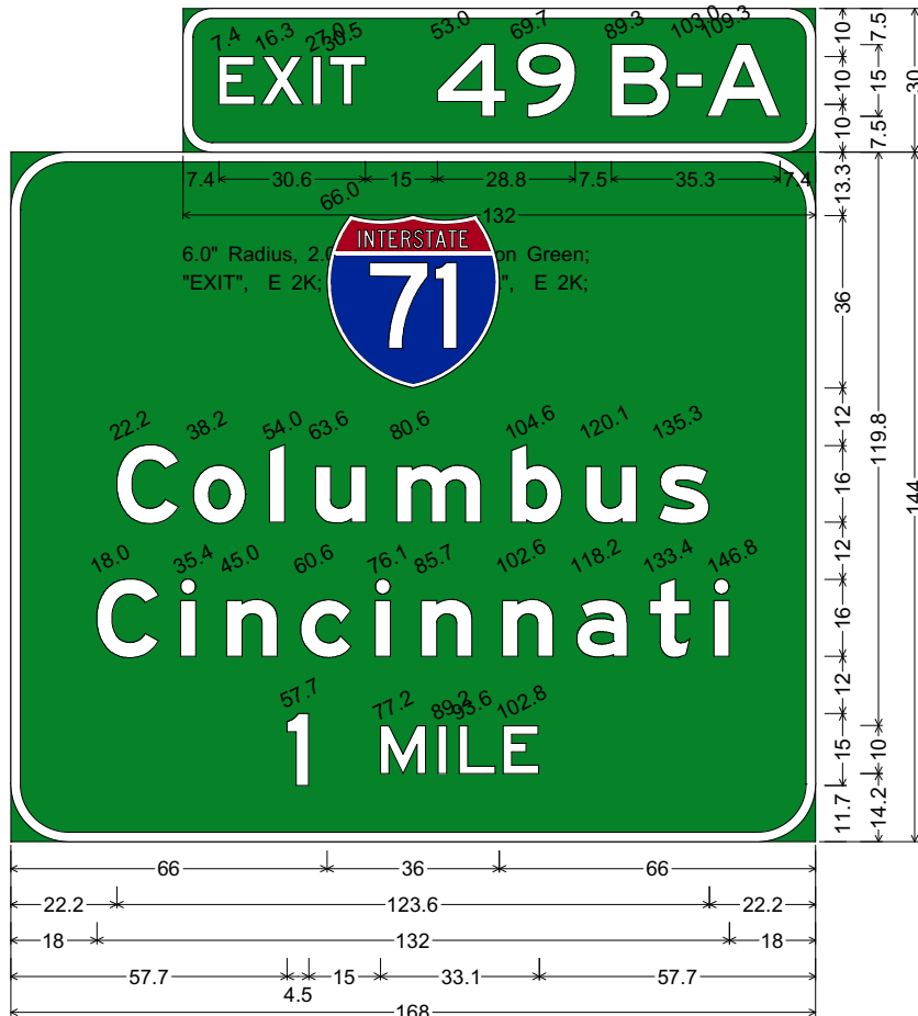
12.0" Radius, 2.0" Border, White on Green; Interstate 71 M1-1; "Columbus", E Mod 2K; "Cincinnati", E Mod 2K; "1 MILE", E 2K;
