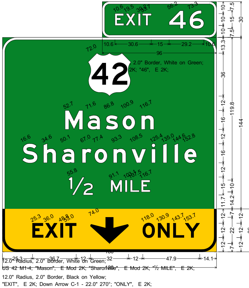
12.0" Radius, 2.0" Border, White on Green; US 42 M1-4; "Mason", E Mod 2K; "Sharonville", E Mod 2K; "1/2 MILE", E 2K;
