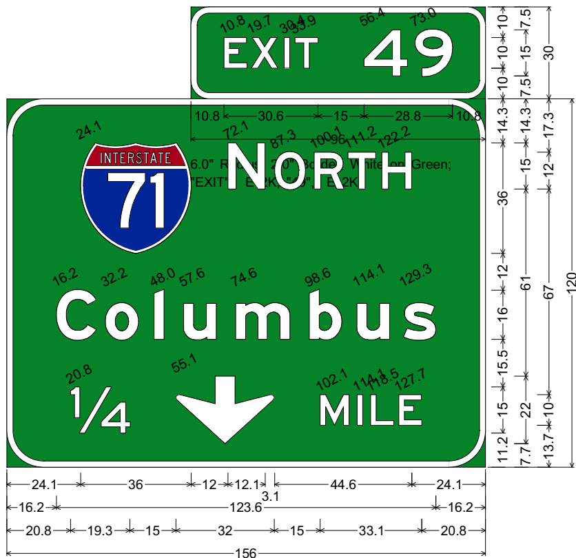
12.0" Radius, 2.0" Border, White on Green; Interstate 71 M1-1; "NORTH", E 2K; "Columbus", E Mod 2K; "1/4", E 2K; Down Arrow C-1 - 22.0" 270°; "MILE", E 2K;
