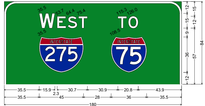
12.0" Radius, 2.0" Border, White on Green; "WEST", E 2K; "TO", E 2K; Interstate 275 M1-1; Interstate 75 M1-1;
