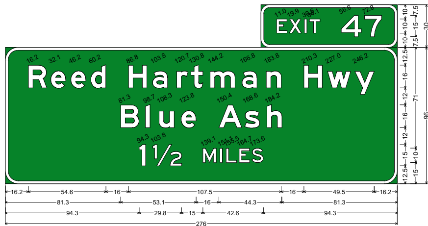
9.0" Radius, 2.0" Border, White on Green; "Reed Hartman Hwy", E Mod 2K; "Blue Ash", E Mod 2K; "1 1/2 MILES", E 2K;
