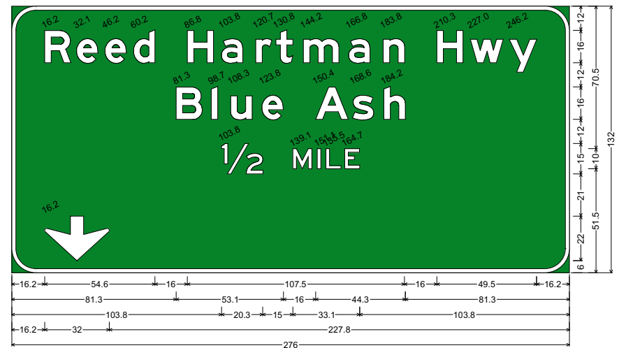
12.0" Radius, 2.0" Border, White on Green; "Reed Hartman Hwy", E Mod 2K; "Blue Ash", E Mod 2K; "1/2 MILE", E 2K; Down Arrow C-1 - 22.0" 270";
