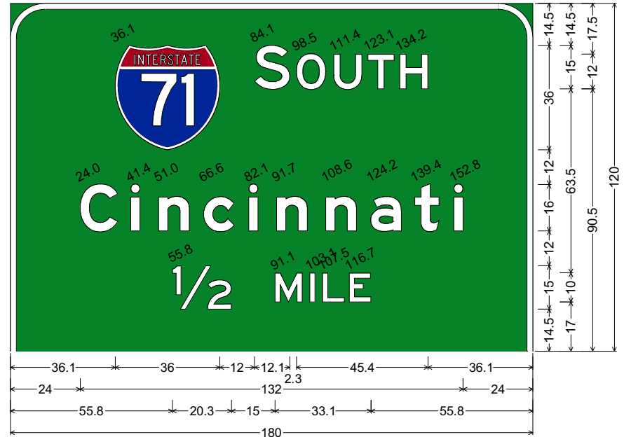
12.0" Radius, 2.0" Border, White on Green; Interstate 71 M1-1; "SOUTH", E 2K; "Cincinnati", E Mod 2K; "1/2 MILE", E 2K;
