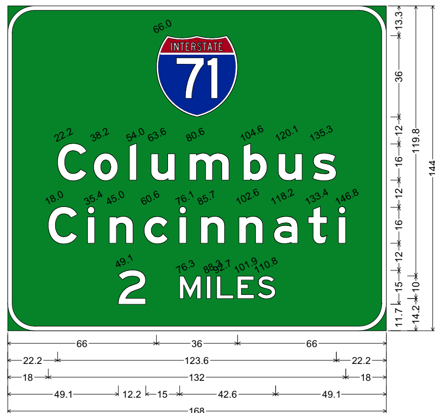
12.0" Radius, 2.0" Border, White on Green; Interstate 71 M1-1; "Columbus", E Mod 2K; "Cincinnati", E Mod 2K; "2 MILES", E 2K;
