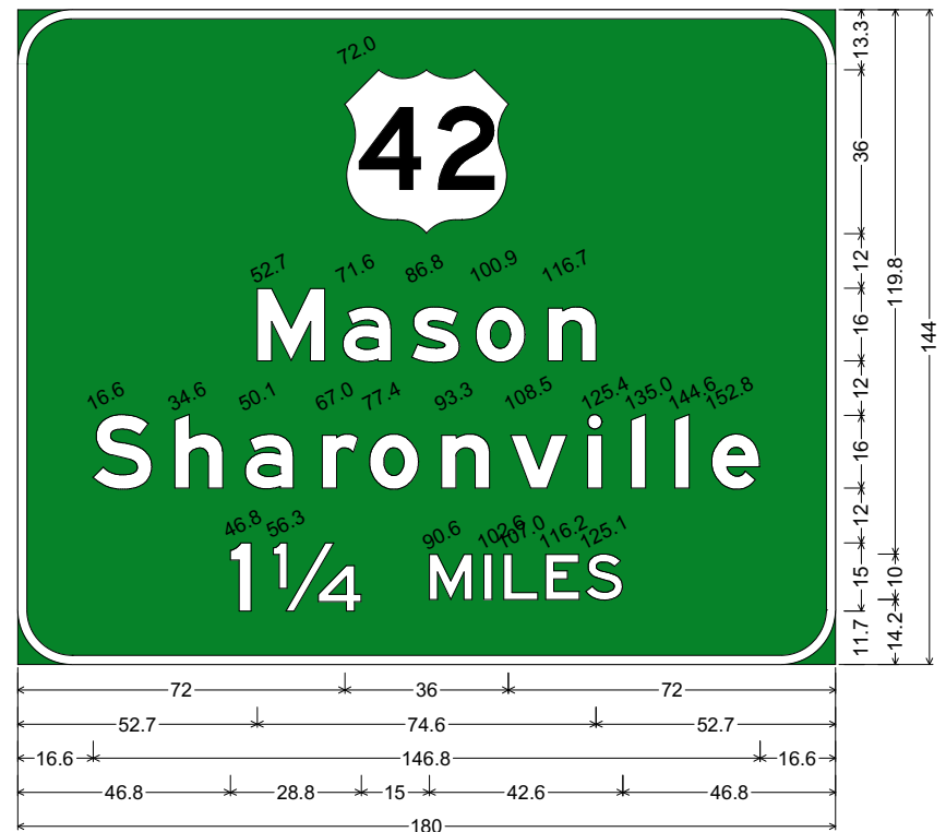
12.0" Radius, 2.0" Border, White on Green; US 42 M1-4; "Mason", E Mod 2K; "Sharonville", E Mod 2K; "1/4 MILES", E 2K;
