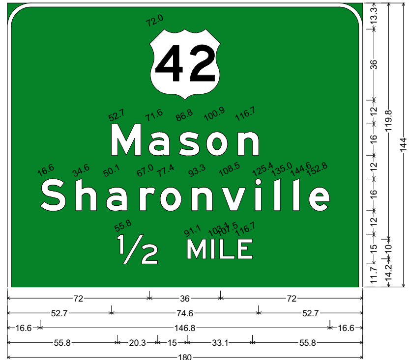
12.0" Radius, 2.0" Border, White on Green; US 42 M1-4; "Mason", E Mod 2K; "Sharonville", E Mod 2K; "1/2 MILE", E 2K;
