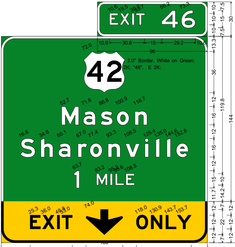
12.0" Radius, 2.0" Border, White on Green; US 42 M1-4; "Mason", E Mod 2K; "Sharonville", E Mod 2K; "1 MILE", E 2K; 12.0" Radius, 2.0" Border, Black on Yellow; "EXIT", E 2K; Down Arrow C-1 - 22.0" 270°; "ONLY", E 2K;
