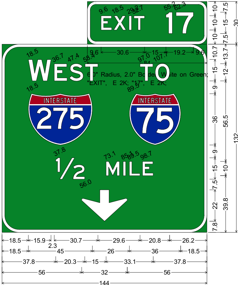
12.0" Radius, 2.0" Border, White on Green; "WEST", E 2K; "TO", E 2K; Interstate 275 M1-1; Interstate 75 M1-1; "1/2", E 2K; "MILE", E 2K; Down Arrow C-1 - 22.0" 270°;
