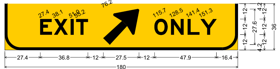
12.0" Radius, 2.0" Border, Black on Yellow; "EXIT", E 2K; Arrow A-1 - 35.0" 45°; "ONLY", E 2K;
