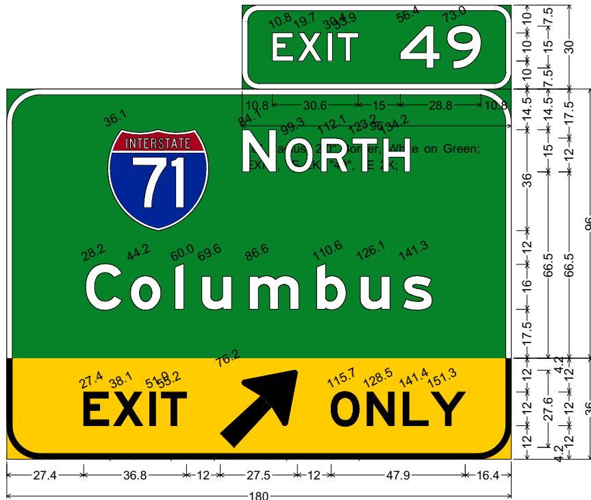
12.0" Radius, 2.0" Border, Black on Yellow; "EXIT", E 2K; Arrow A-1 - 35.0° 45°; "ONLY", E 2K;
