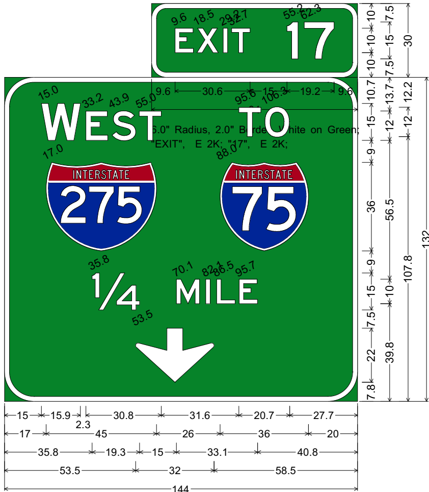
12.0" Radius, 2.0" Border, White on Green; "WEST", E 2K; "TO", E 2K; Interstate 275 M1-1; Interstate 75 M1-1; "1/4", E 2K; "MILE", E 2K; Down Arrow C-1 - 22.0" 270°;
