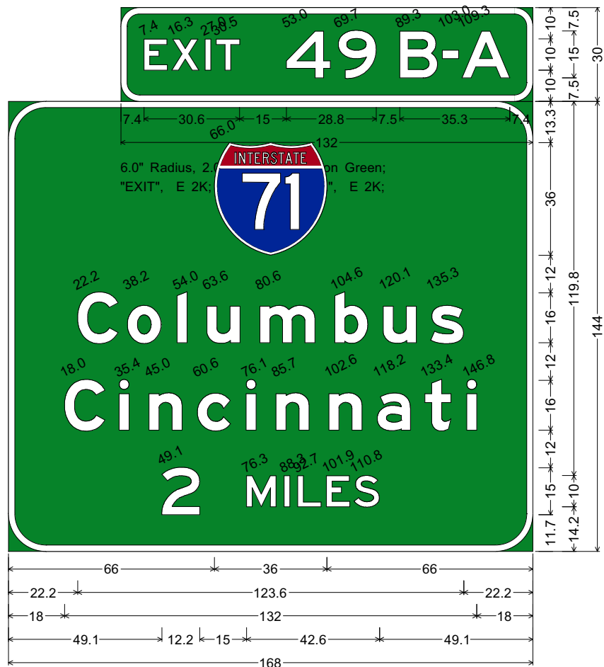
12.0" Radius, 2.0" Border, White on Green; Interstate 71 M1-1; "Columbus", E Mod 2K; "Cincinnati", E Mod 2K; "2 MILES", E 2K;
