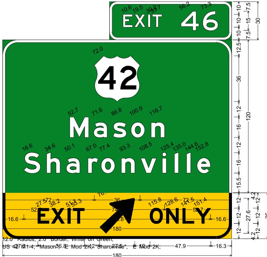
12.0" Radius, 2.0" Border, Black on Yellow; "EXIT", E 2K; Arrow A-1 - 35.0" 45"; "ONLY", E 2K;
