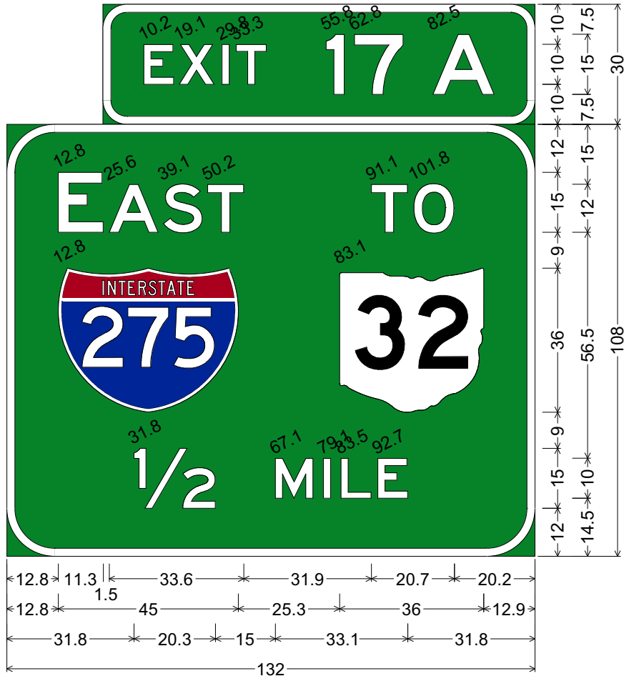
12.0" Radius, 2.0" Border, White on Green; "EAST", E 2K; "TO", E 2K; Interstate 275 M1-1; State Highway 32 M1-H5-36-2; "1/2 MILE", E 2K;
