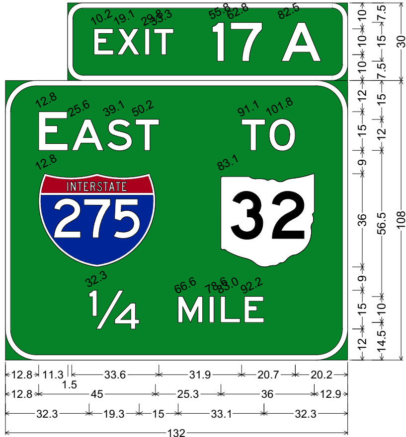
12.0" Radius, 2.0" Border, White on Green; "EAST", E 2K; "TO", E 2K; Interstate 275 M1-1; State Highway 32 M1-H5-36-2; "1/4 MILE", E 2K;
