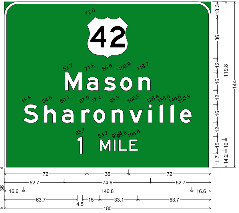
12.0" Radius, 2.0" Border, White on Green; US 42 M1-4; "Mason", E Mod 2K; "Sharonville", E Mod 2K; "1 MILE", E 2K;
