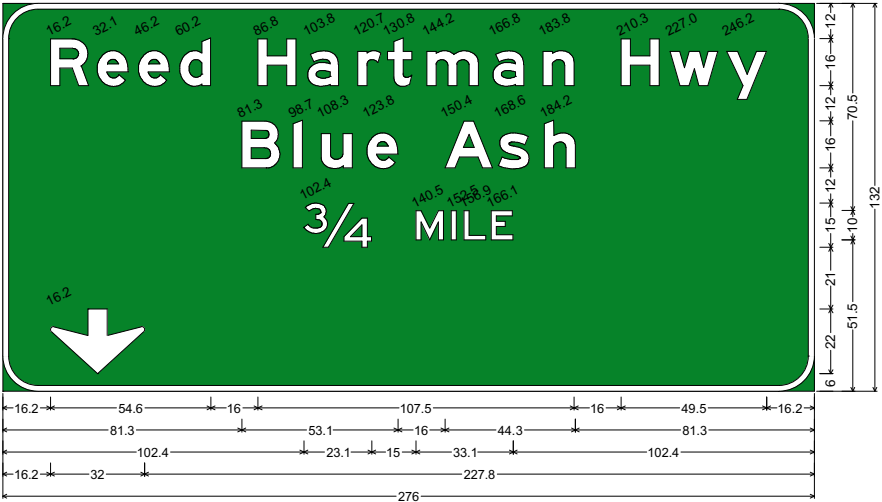
12.0" Radius, 2.0" Border, White on Green; "Reed Hartman Hwy", E Mod 2K; "Blue Ash", E Mod 2K; "3/4 MILE", E 2K; Down Arrow C-1 - 22.0" 270";
