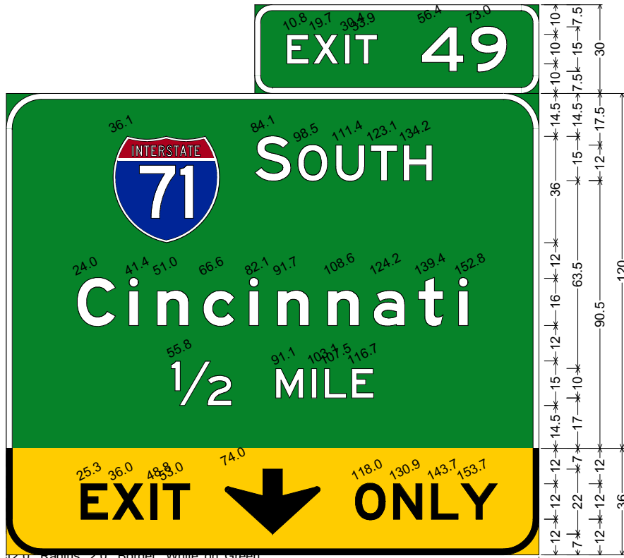
12.0" Radius, 2.0" Border, White on Green; Interstate 71 M1-1; "SOUTH", E 2K; "Cincinnati", E Mod 2K; "1/2", E 2K; "MILE", E 2K; "", E 2K;
