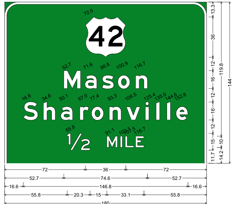
12.0" Radius, 2.0" Border, White on Green; US 42 M1-4; "Mason", E Mod 2K; "Sharonville", E Mod 2K; "1/2 MILE", E 2K;
