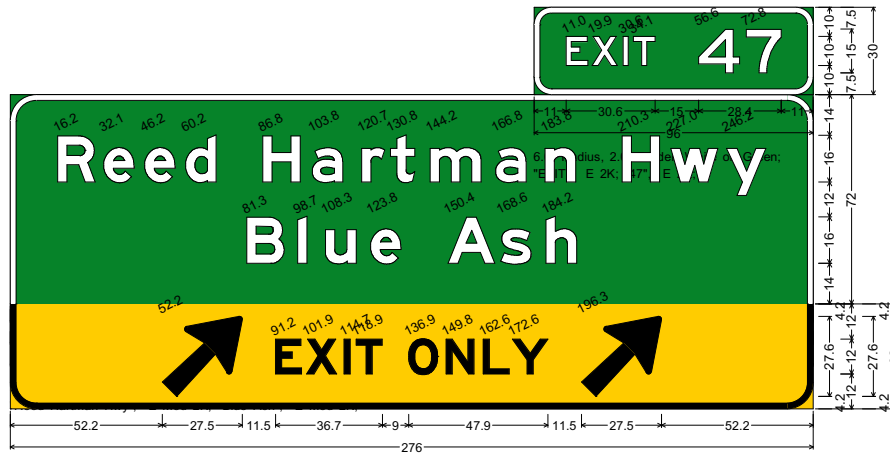
9.0" Radius, 2.0" Border, Black on Yellow; Arrow A-1 - 35.0° 45°; "EXIT", E 2K; "ONLY", E 2K; Arrow A-1 - 35.0° 45°;
