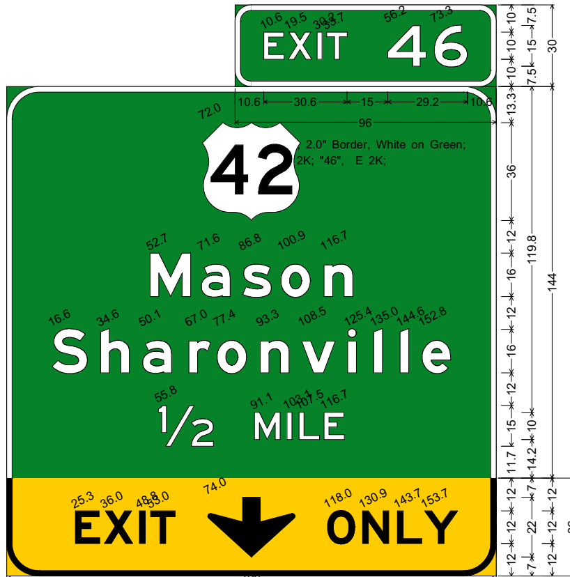
12.0" Radius, 2.0" Border, White on Green; US 42 M1-4, "Mason", E Mod 2K, "Sharonville", E Mod 2K, "1/2 MILE", E 2K; 12.0" Radius, 2.0" Border, Black on Yellow; "EXIT", E 2K; Down Arrow C-1 - 22.0" 270"; "ONLY", E 2K;
