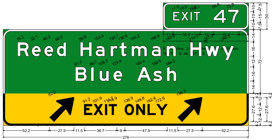
9.0" Radius, 2.0" Border, Black on Yellow; Arrow A-1 - 35.0° 45°; "EXIT", E 2K; "ONLY", E 2K; Arrow A-1 - 35.0° 45°;
