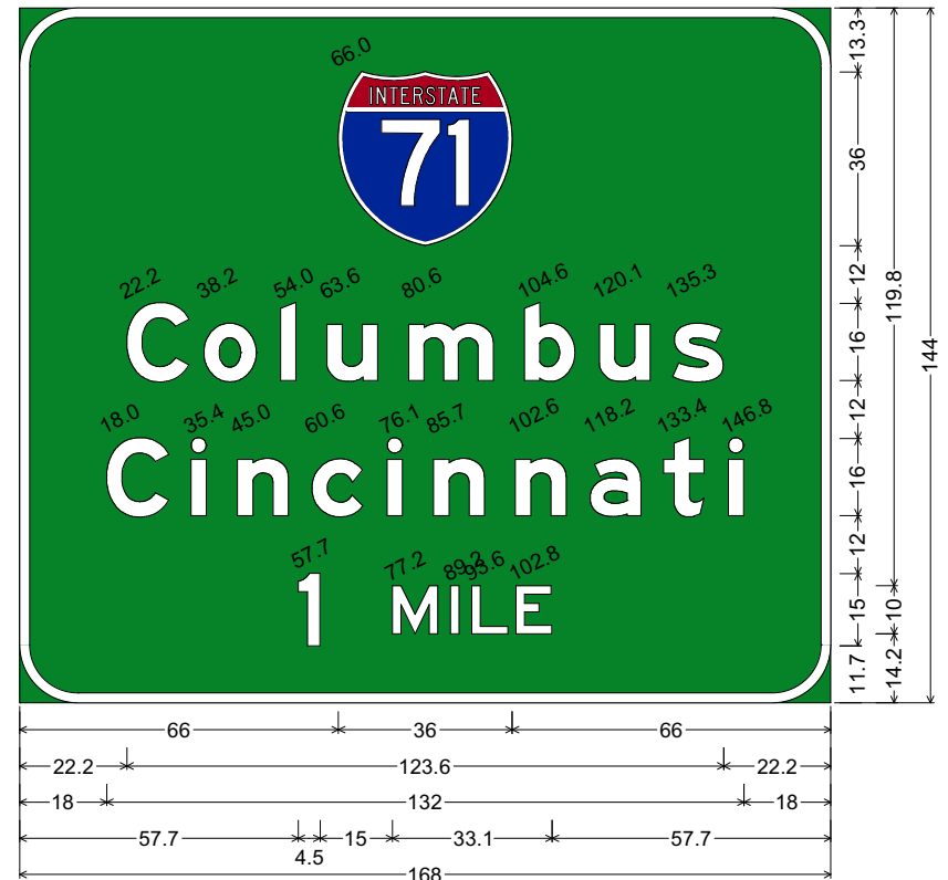
12.0" Radius, 2.0" Border, White on Green; Interstate 71 M1-1; "Columbus", E Mod 2K; "Cincinnati", E Mod 2K; "1 MILE", E 2K;
