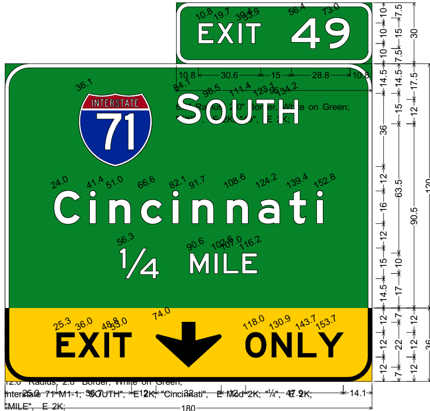
12.0" Radius, 2.0" Border, Black on Yellow; "EXIT", E 2K; Down Arrow C-1 - 22.0" 270°; "ONLY", E 2K;
