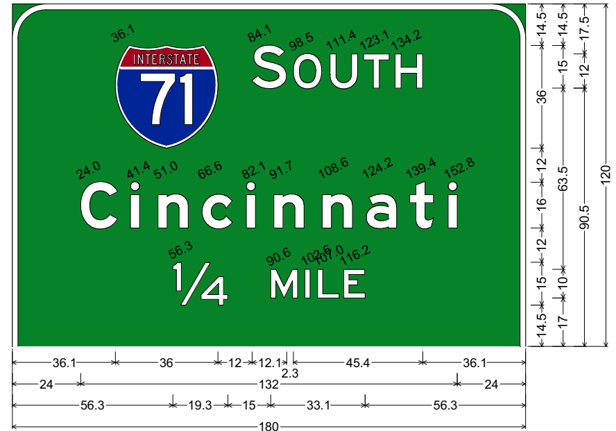
12.0" Radius, 2.0" Border, White on Green; Interstate 71 M1-1; "SOUTH", E 2K; "Cincinnati", E Mod 2K; "1/4", E 2K; "MILE", E 2K;
