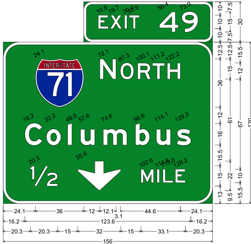
12.0" Radius, 2.0" Border, White on Green; Interstate 71 M1-1; "NORTH", E 2K; "Columbus", E Mod 2K; "1/2", E 2K; Down Arrow C-1 - 22.0° 270°; "MILE", E 2K;
