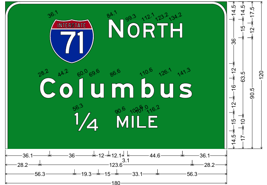
12.0" Radius, 2.0" Border, White on Green; Interstate 71 M1-1; "NORTH", E 2K; "Columbus", E Mod 2K; "1/4 MILE", E 2K;
