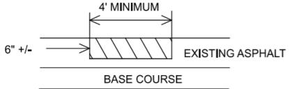
Existing deteriorated asphalt shall be removed to a maximum depth of 6 inches or as directed by the engineer and replace with Item 301, Asphalt Concrete Base, shall be compacted as per 401.15 and in approximately equal layers. The locations and size of the repairs shall be determined by the engineer.
