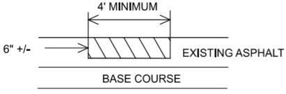
Existing deteriorated asphalt shall be removed to a maximum depth of 6 inches or as directed by the engineer and replace with Item 301, Asphalt Concrete Base, shall be compacted as per 401.15 and in approximately equal layers. The locations and size of the repairs shall be determined by the engineer.
