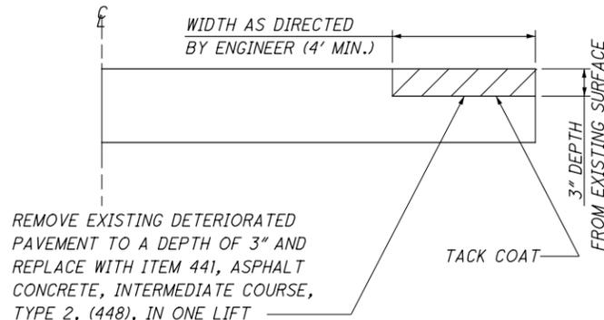
REMOVE EXISTING DETERIORATED PAVEMENT TO A DEPTH OF 3" AND REPLACE WITH ITEM 441, ASPHALT CONCRETE, INTERMEDIATE COURSE, TYPE 2, (448), IN ONE LIFT
