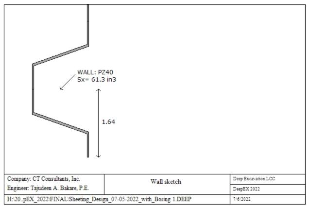
Wall type: Steel sheet piling
