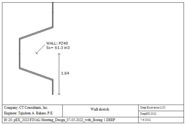
Wall type: Steel sheet piling
