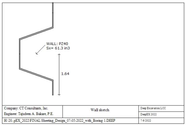
Wall type: Steel sheet piling
