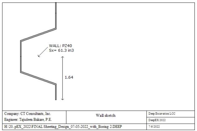
Wall type: Steel sheet piling
