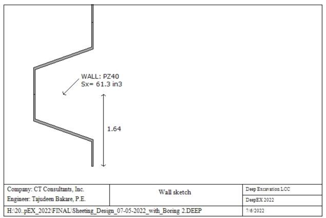
Wall type: Steel sheet piling
