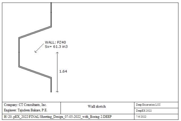
Wall type: Steel sheet piling
