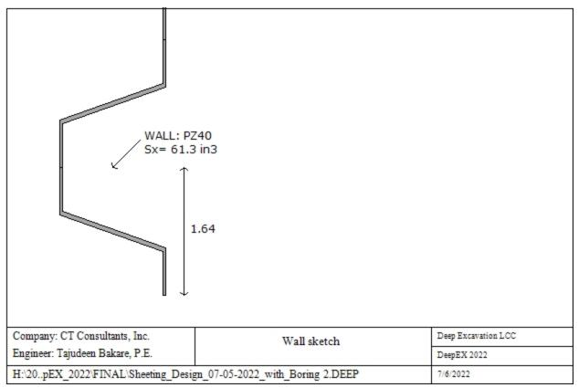
Wall type: Steel sheet piling
