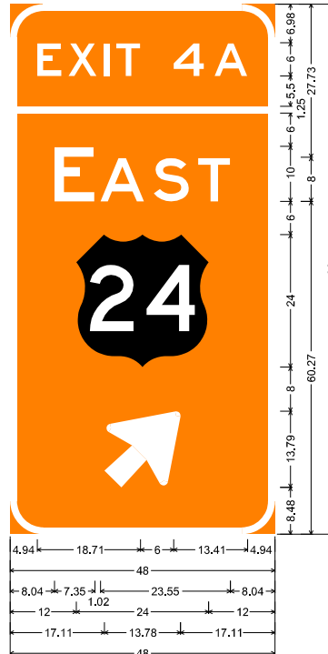
SN-102, SN-108, SN-113, SN-114, SN-124 6.00" Radius, 1.25" Border, Black on Orange; [EXIT 4A] E: [E]; [AST] E: US 24 M1-4; Arrow B-4 - 17.00" 45°;
