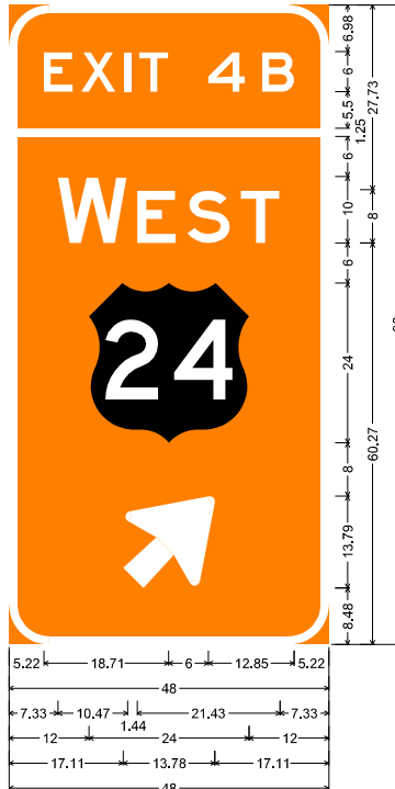
SN-103, SN-115, SN-125 6.00" Radius, 1.25" Border, Black on Orange; [EXIT 4B] E: [W] E; [E] E; US 24 M1-4; Arrow B-4 - 17.00" 45°;
