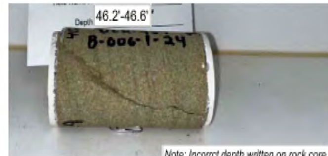
Note: Incorrect depth written on rock core
