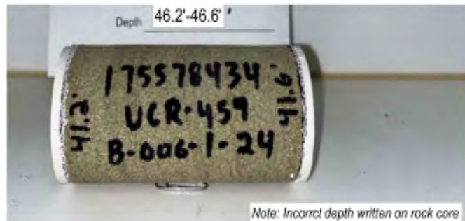
Note: Incorrect depth written on rock core
