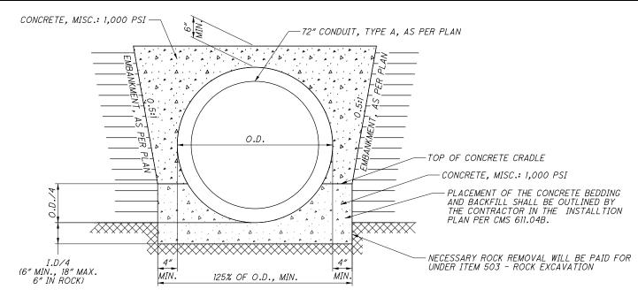
CONCRETE BACKFILL AND BEDDING DETAIL
