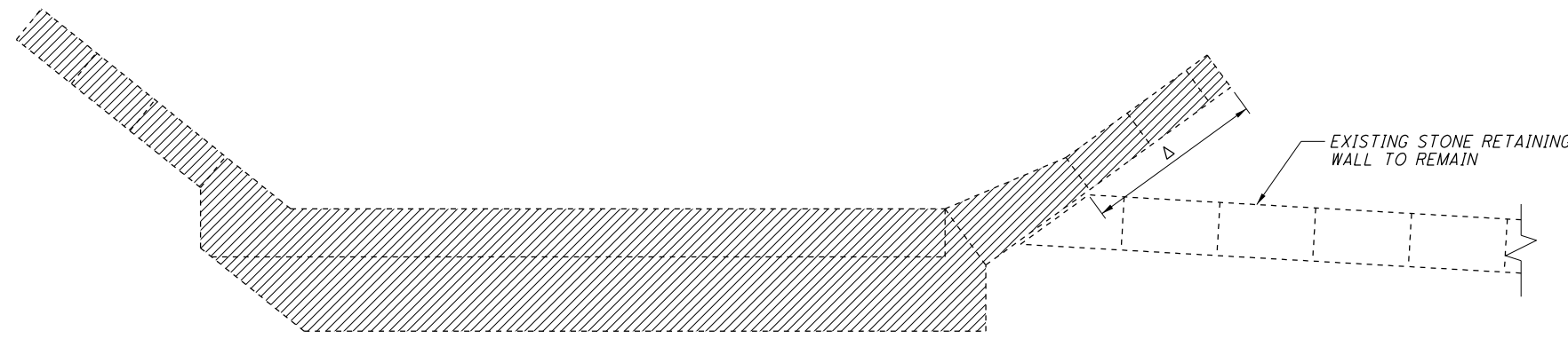
ABUTMENT REMOVAL PLAN
