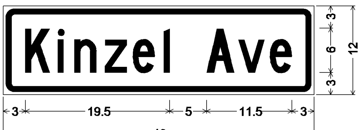
1.5" Radius, 0.8" Border, 0.4" Indent, White on Green; [Kinzel] C 75% spacing; [Ave] C 75% spacing;
