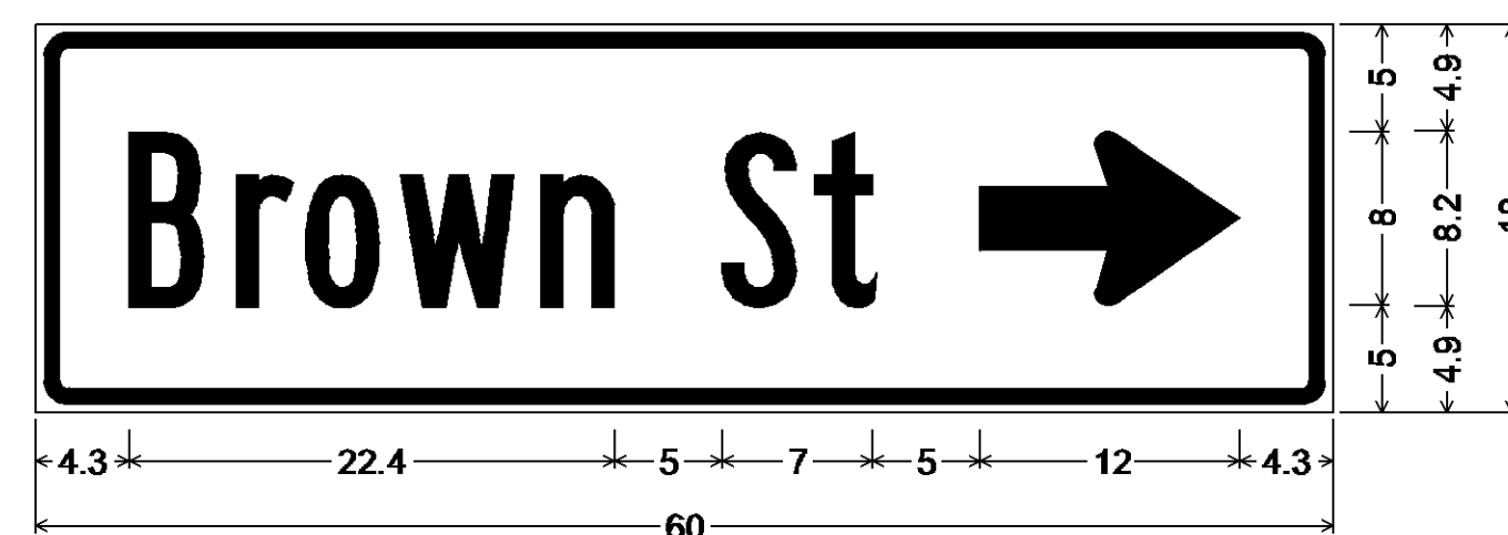
1.5" Radius, 0.8" Border, 0.4" Indent, White on Green; [Brown] B 75% spacing; [St] B 75% spacing; Standard Arrow Custom 12.0" X 8.1" 0°;
