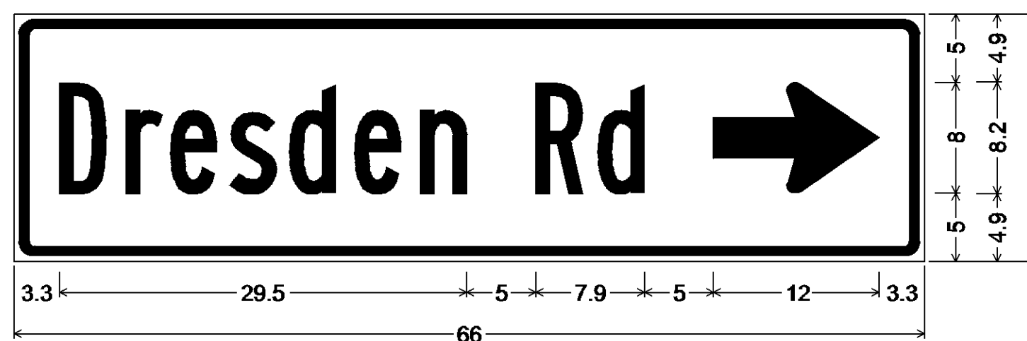
1.5" Radius, 0.8" Border, 0.4" Indent, White on Green; [Dresden] B 75% spacing; [Rd] B 75% spacing; Standard Arrow Custom 12.0" X 8.1" 0°;
