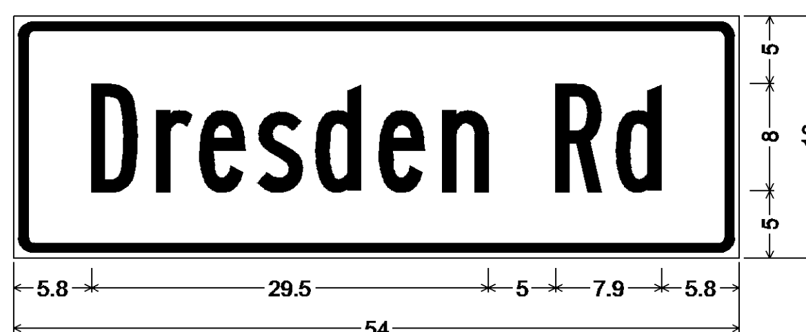
1.5" Radius, 0.8" Border, 0.4" Indent, White on Green; [Dresden] B 75% spacing; [Rd] B 75% spacing;
