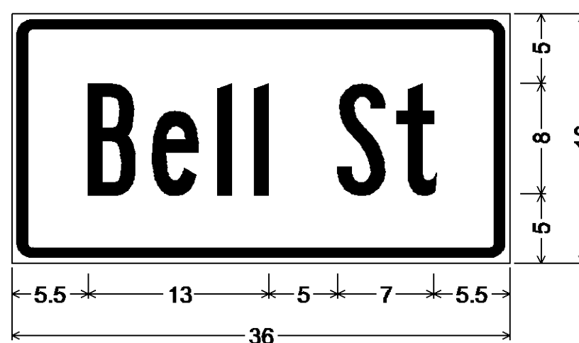
1.5" Radius, 0.8" Border, 0.4" Indent, White on Green; [Bell] B 75% spacing; [St] B 75% spacing;
