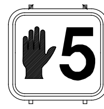
PEDESTRIAN HEADS (LED, COUNTDOWN, TYPE D2)
