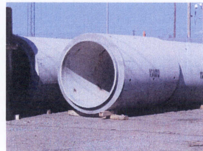
Reinf. Conc. Jacking Pipe
