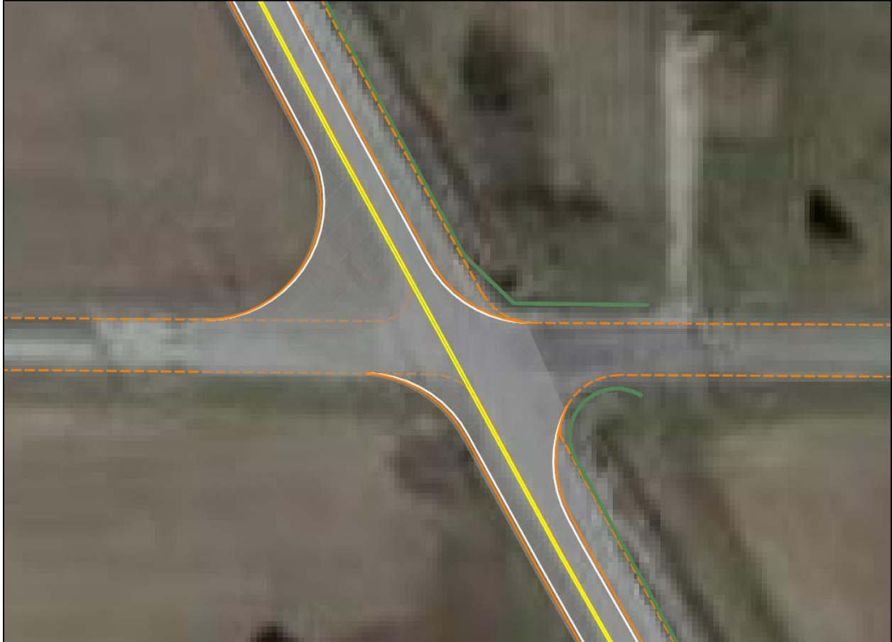
Close-up of conceptual drawing of SR-64 realignment. The new alignment is shown in solid lines and shaded in gray. The current roadway is shown with orange dashed lines. The guardrail runs are shown with green lines.
