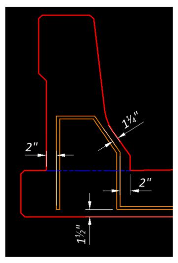
C&MS 509.04.D – Placement tolerance from the surface is  $(-0^{\circ}, +1/2^{\circ})$
