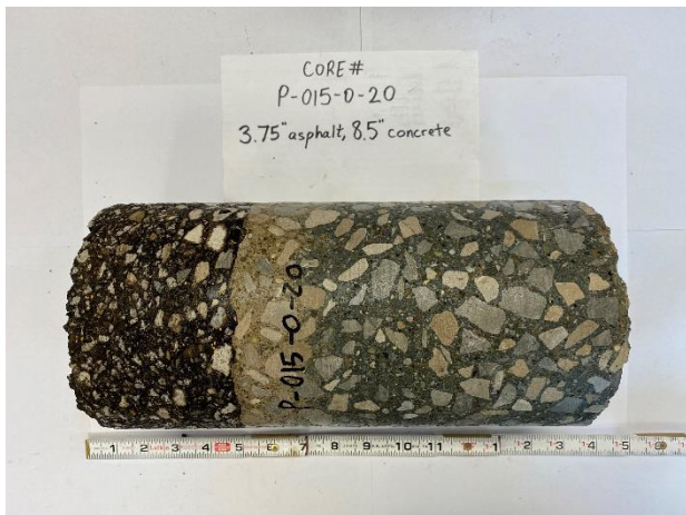
Project Name: SUM 76-77 Phase 3 Retaining Wall on SR8 Project Number: 1822-1016-00 Boring: P-015-0-20 Asphalt: 3.75" Concrete: 8.5" Date Cored: 06/30/2020 Date Drilled: 06/30/2020
