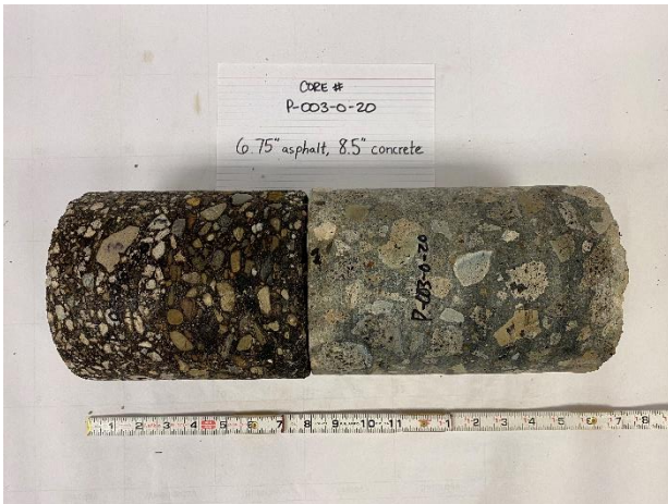
Project Name: SUM 76-77 Phase 3 Retaining Wall on SR8 Project Number: 1822-1016-00 Boring: P-003-0-20 Asphalt: 6.75" Concrete: 8.5" Date Cored: 06/24/2020 Date Drilled: 06/25/2020
