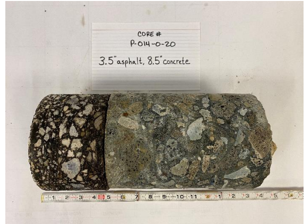
Project Name: SUM 76-77 Phase 3 Retaining Wall on SR8 Project Number: 1822-1016-00 Boring: P-014-0-20 Asphalt: 3.5" Concrete: 8.5" Date Cored: 06/25/2020 Date Drilled: 06/25/2020
