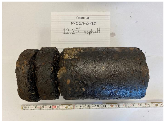
Project Name: SUM 76-77 Phase 3 Retaining Wall on SR8 Project Number: 1822-1016-00 Boring: P-027-0-20 Asphalt: 12.25" Concrete: Date Cored: 06/30/2020 Date Drilled: 07/01/2020
