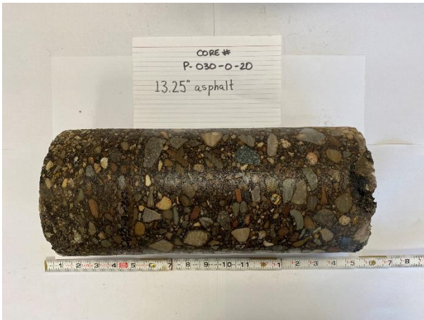
Project Name: SUM 76-77 Phase 3 Retaining Wall on SR8 Project Number: 1822-1016-00 Boring: P-030-0-20 Asphalt: 13.25" Concrete: Date Cored: 07/01/2020 Date Drilled: 07/01/2020
