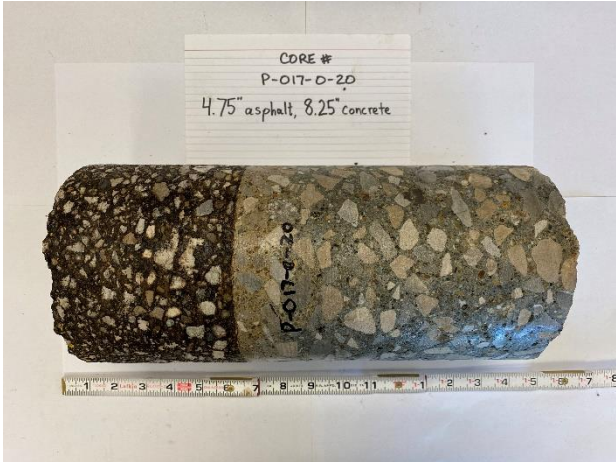
Project Name: SUM 76-77 Phase 3 Retaining Wall on SR8 Project Number: 1822-1016-00 Boring: P-017-0-20 Asphalt: 4.75" Concrete: 8.25" Date Cored: 06/30/2020 Date Drilled: 06/30/2020
