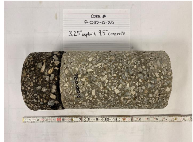
Project Name: SUM 76-77 Phase 3 Retaining Wall on SR8 Project Number: 1822-1016-00 Boring: P-010-0-20 Asphalt: 3.25" Concrete: 9.5" Date Cored: 06/25/2020 Date Drilled: 06/25/2020
