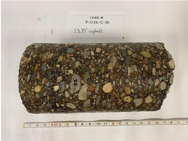
Project Name: SUM 76-77 Phase 3 Retaining Wall on SR8 Project Number: 1822-1016-00 Boring: P-022-0-20 Asphalt: 13.75" Concrete: Date Cored: 06/23/2020 Date Drilled: 06/23/2020
