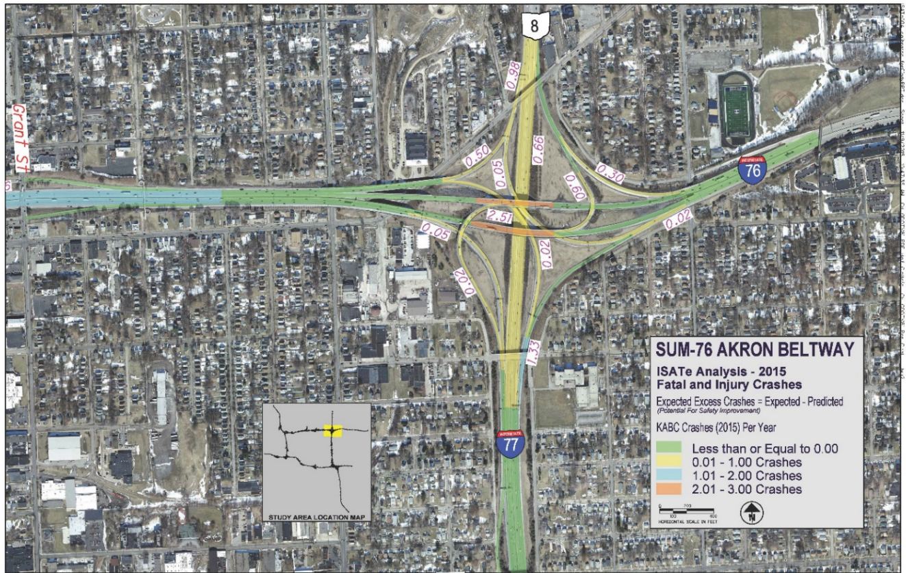
Figure 12 – Northeast (Central) Interchange Expected and Predicted Crashes
