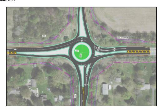
During the DSRT stakeholder presentation, concerns were raised regarding the two westbound through lanes entering the roundabout and the subsequent lane reduction. ODOT'S ECAT cannot account for the lane reduction downstream of the roundabout. Results were thought to be misleading. Stakeholders felt that capacity was being prioritized over safety.
