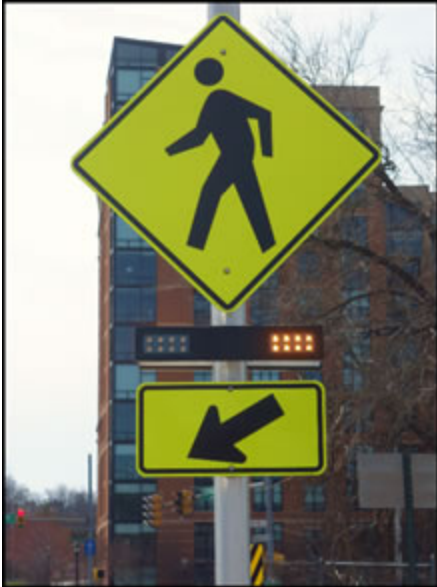
Figure 1. Example of an RRFB dark (left) and illuminated during the flash period (center and right) mounted with W11-2 sign and W16-7P plaque at an uncontrolled marked crosswalk.
