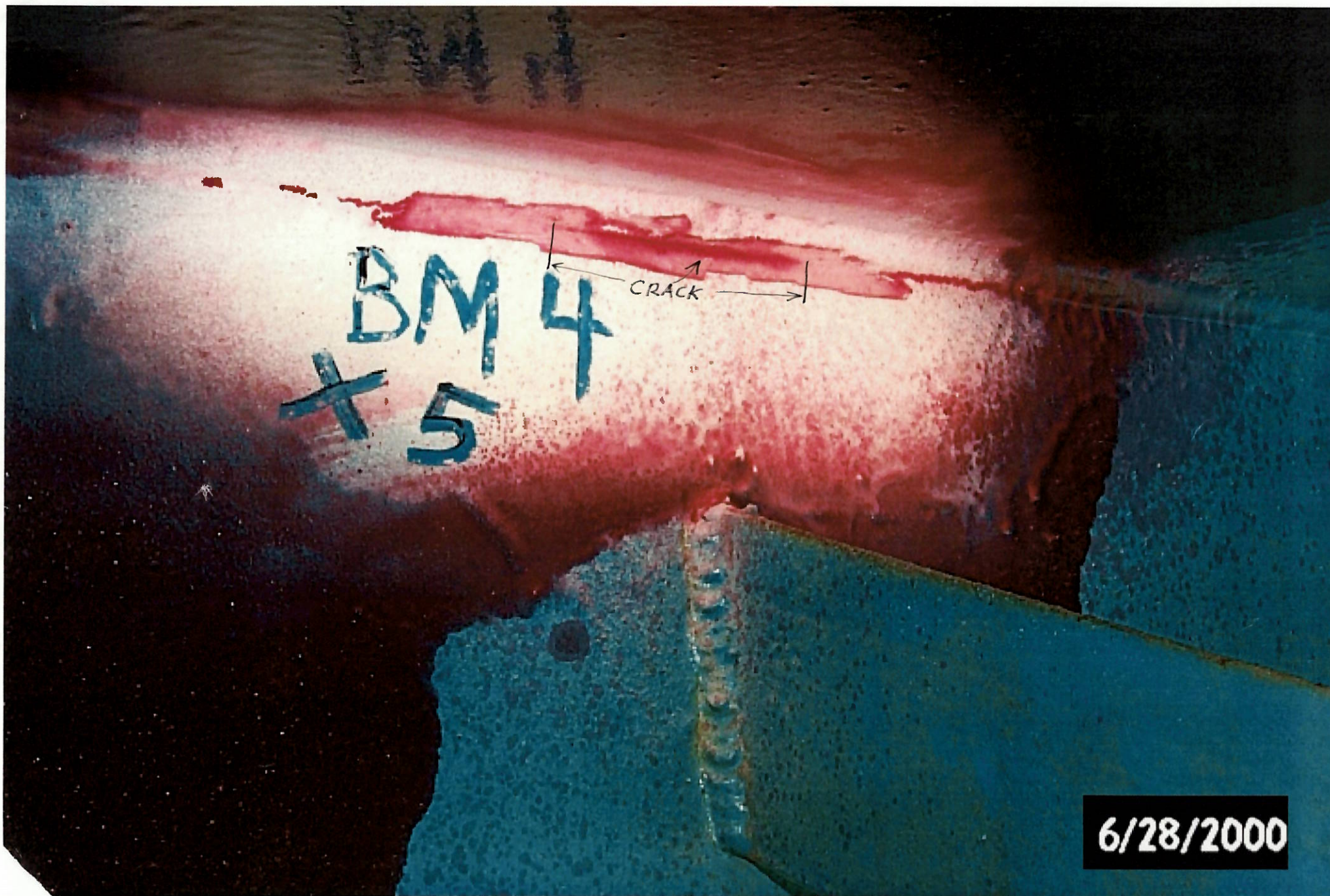
CRACK LOCATION #2 AFTER DYE PENETRANT TEST
