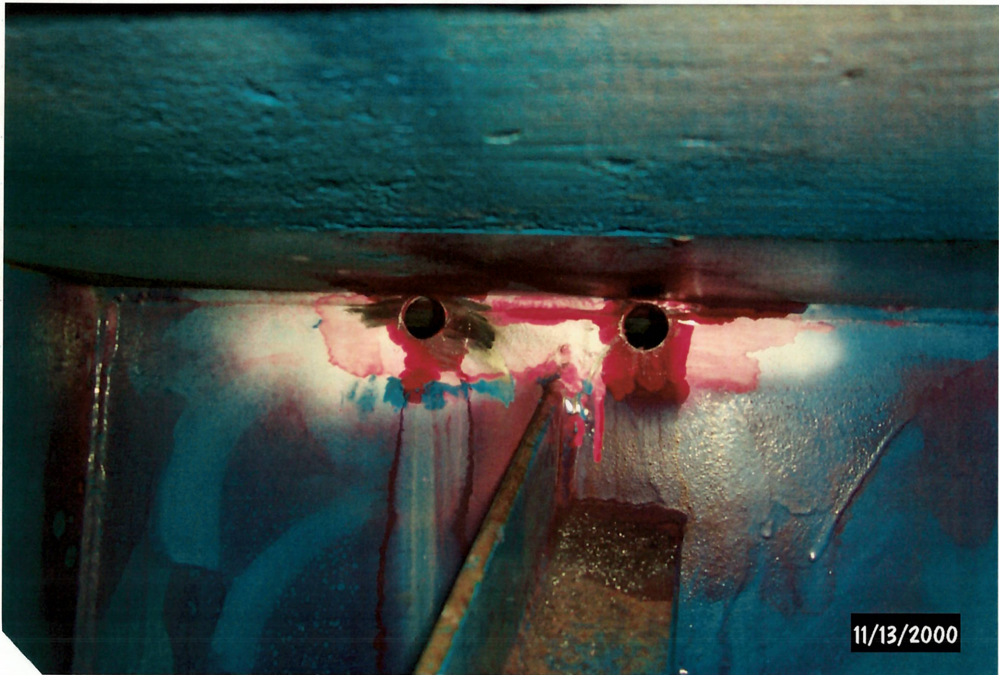
CRACK LOCATION #3 AFTER 3/4" HOLES DRILLED
