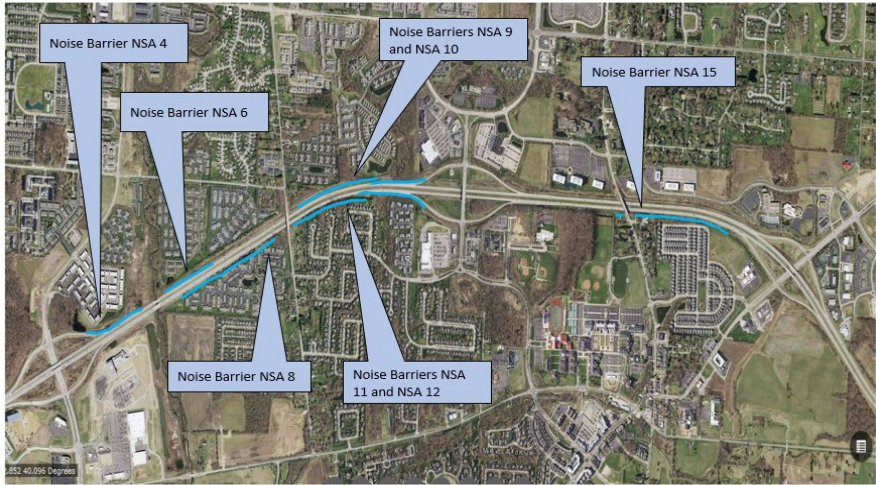
Figure 11 Recommended Noise Barrier Wall Locations FRA-161-15.85 PID 116322
