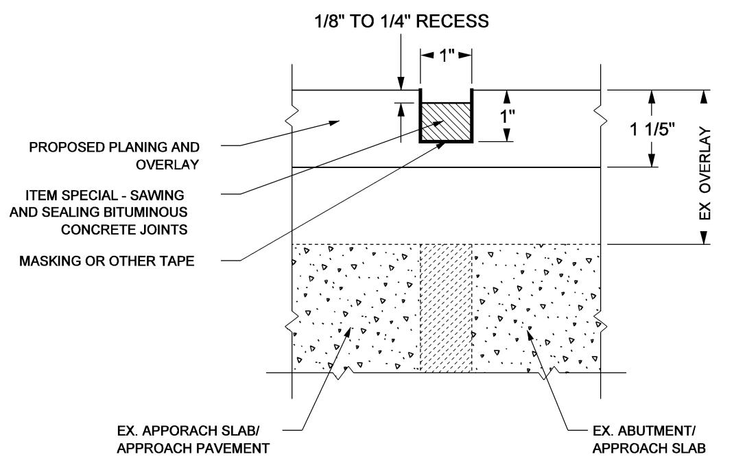
NOTE: THE CONTRACTOR SHALL MARK THE, EXISTING APPROACH SLAB JOINT PRIOR TO WORK TO ASSURE THE JOINT SAWING AND SEALING WILL BE PROPERLY PLACED.
