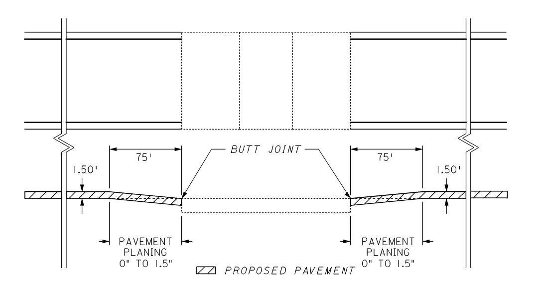
ITEM 254 - PAVEMENT PLANING, ASPHALT CONCRETE: PLANING TO BE USED AT THE STRUCTURES.
