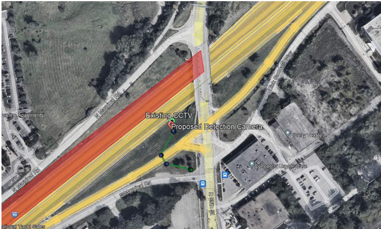
Figure 67: QWS-OVRHD-D12-I-90_WB AT DOWNTOWN Existing DMS and structure to be replaced with new full-color DMS and new truss structure. Proposed detection camera to be attached to new DMS truss structure
