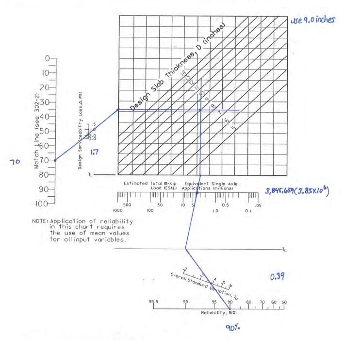
Rigid parement design for Groves Rd (East) as per markings from CUC
