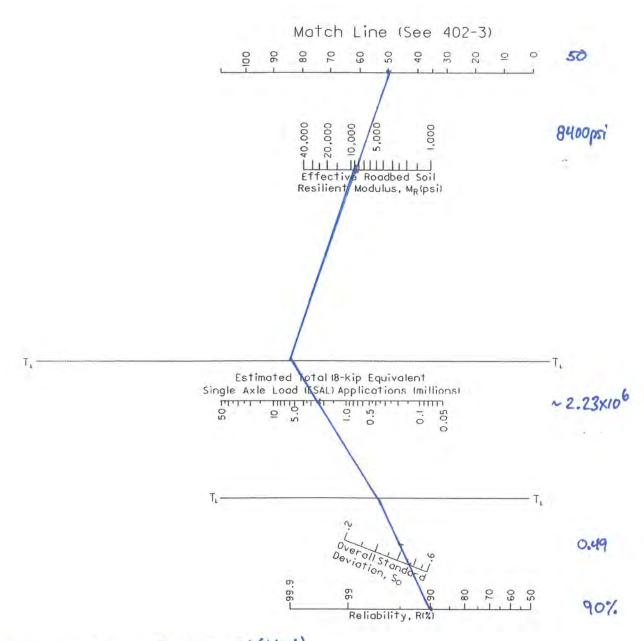
Flexible pavement design for Groves Rd (West) as per mortcups from COC
