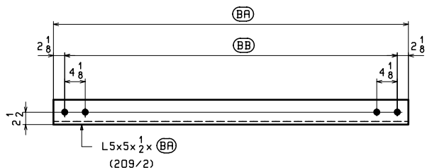
CROSSFRAME TOP & BTM STRUTS ~ MARK "A" (209/2)
