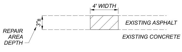
EXISTING DETERIORATED ASPHALT SHALL BE REMOVED TO A DEPTH OF 3"± AND MINIMUM WIDTH OF 4' OR AS DIRECTED BY THE ENGINEER. THIS WORK CONSISTS OF PARTIAL DEPTH REMOVAL OF EXISTING PAVEMENT IN AREAS EXHIBITING DETERIORATION AT THE SURFACE, APPLYING TACK COAT, AND PLACING AND COMPACTING ASPHALT CONCRETE. THE LOCATION AND SIZE OF THE REPAIR SHALL BE DETERMINED BY THE ENGINEER. THE EXISTING CONCRETE SURFACE SHALL NOT BE DISTURBED.
