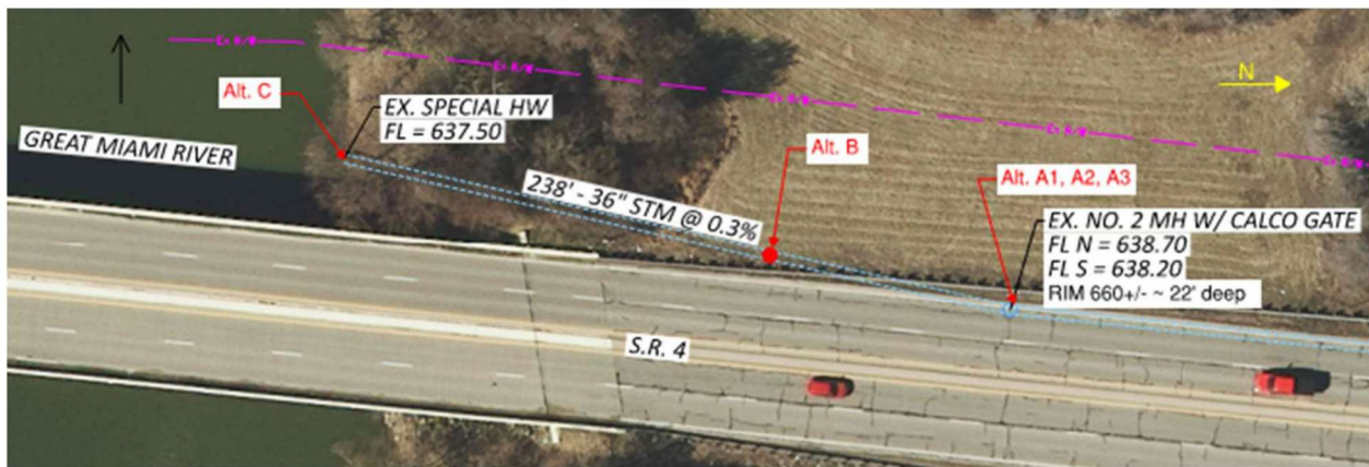
Figure 8: BUT-4 Flap Gate Profile View
