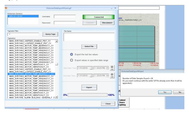
It is necessary to select or create a new text file for the historian data to be exported to. In the example below, the Z: drive is mapped to the NAS system in the server cabinet. A file named test.txt has been seelcted to receive the last ten values.
