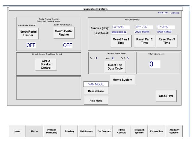
The Circuit Breaker Maintenance screen shows the racked and closed status of each breaker. A trip and closed button can be used to remotely trip a breaker or remotely close a breaker.
