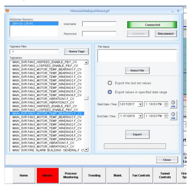
In the example below, the motor bearing 1 temperature is seelected for Fan 3. It is possible to export the historian tag values over a date range, or just the last 10 values.
