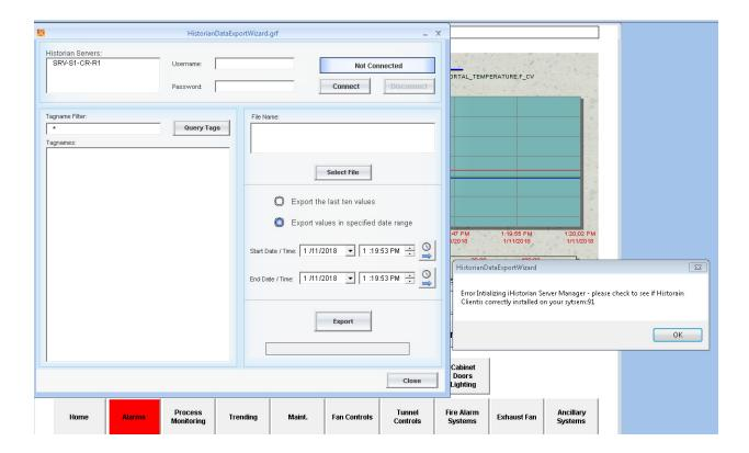
Once the server is connected, the connection indicator will turn green and indicate "Connected". There is a tagname filter that allows for tags to be filtered by name.
