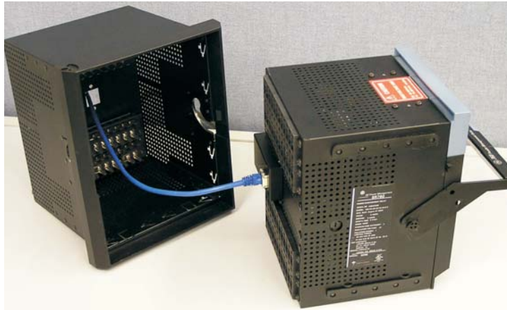
FIGURE 3–10: Ethernet Cable Connection
