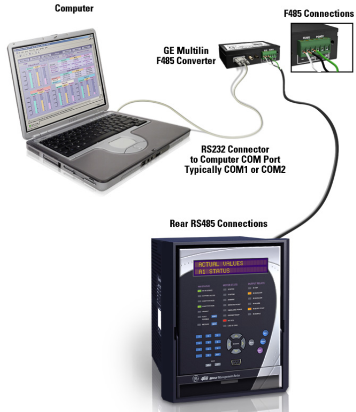
FIGURE 4-3: Communications using Rear RS485 Port
