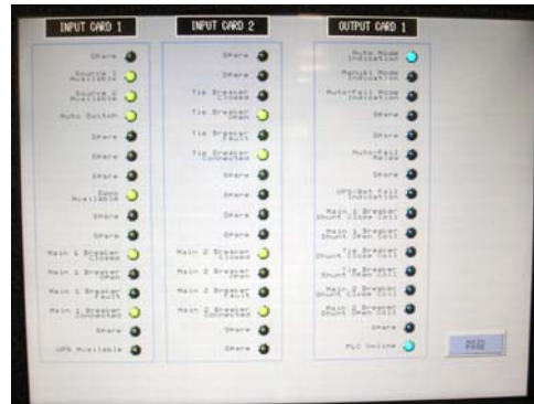
Figure 23: PLC I/O Map Screen
