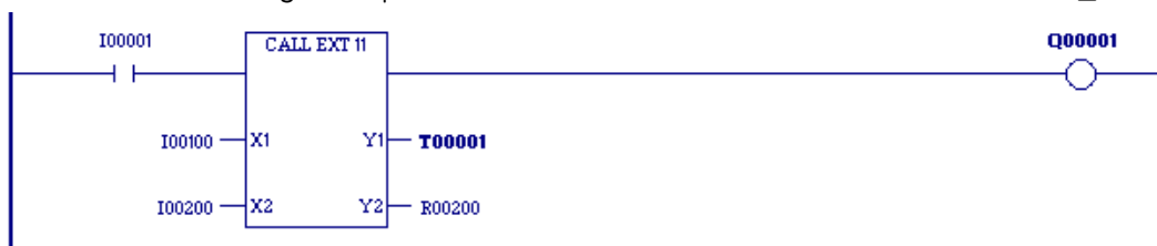
Figure 19: Calling an External Block in Ladder Logic
