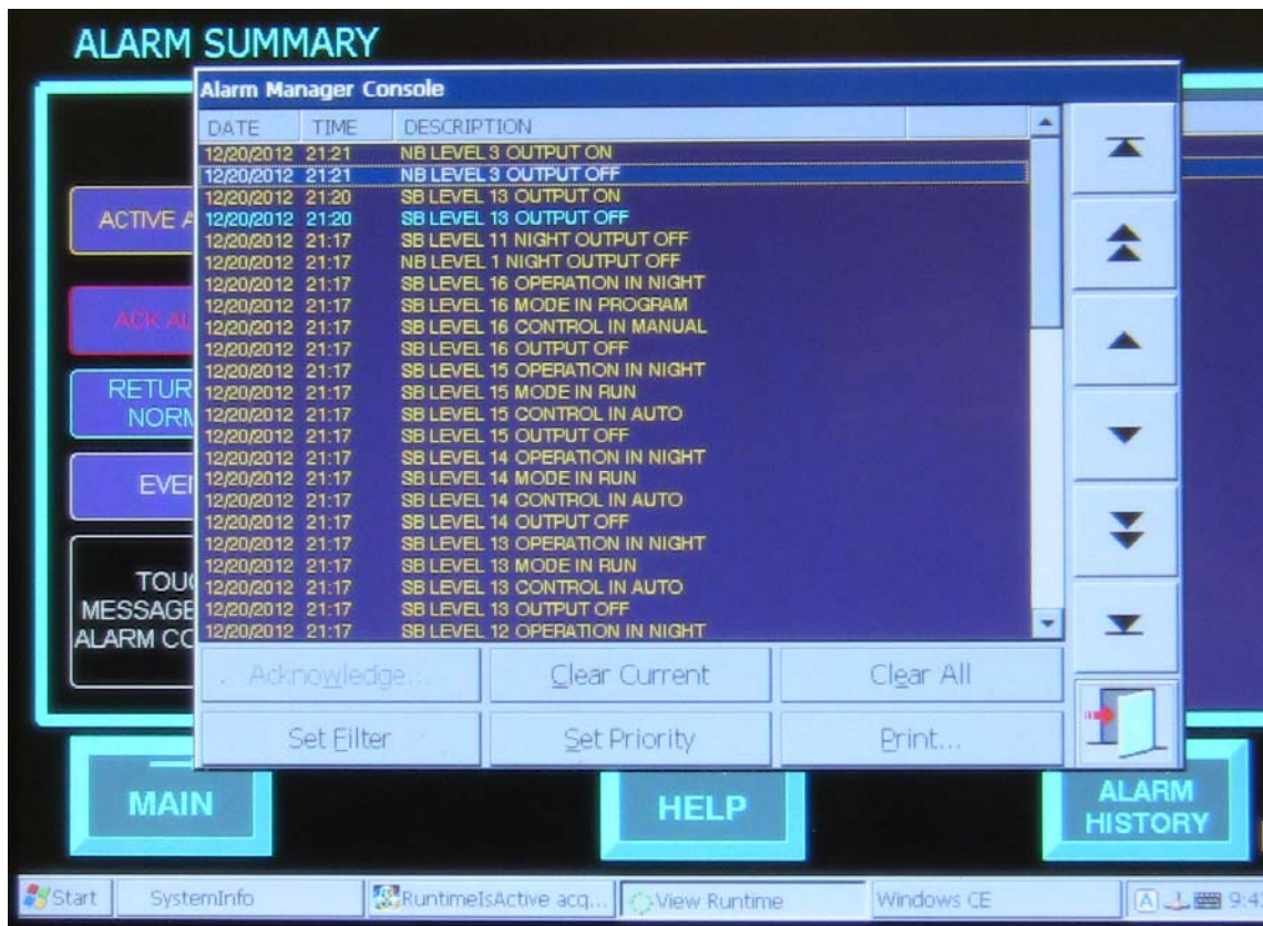
Figure 19.4 Alarm Manager Console
