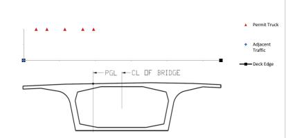
wheel load definition for user-defined vehicle (no need to input data if doing inventory or operating rating using standard HS load configuration)
