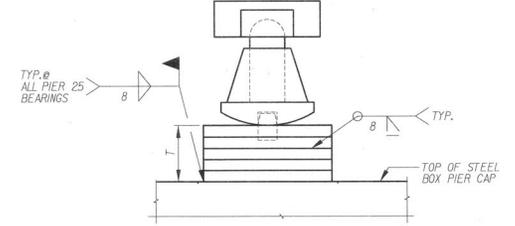
BASE PLATE THICKNESS DETAIL
