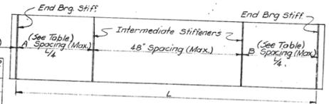
Note: Adjust intermediate stiffener spacing to conform to intermediate crossframe spacing.
