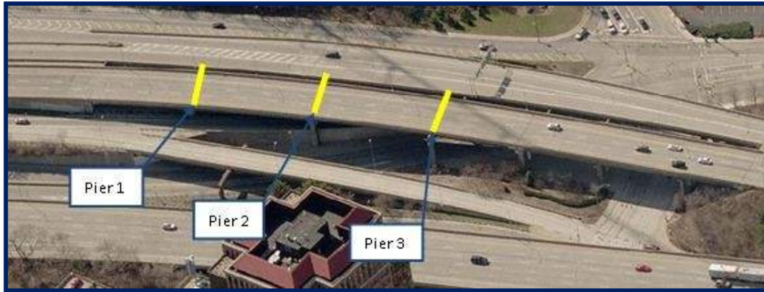
Figure 2: NSTM Pier Cap Locations
