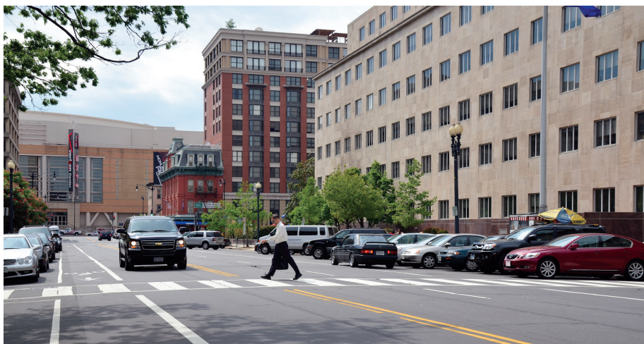
Figure 4-24. Typical Application of Diagonal Back-In/Head-Out Parking
