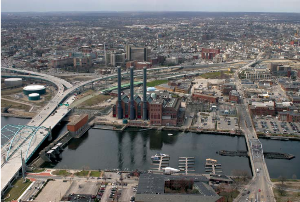
Figure 10-13. Directional Three-Leg Interchange at a River Crossing
