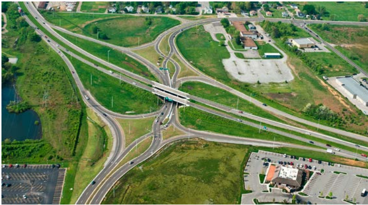
– B – Overpass DDI Source: Tennessee DOT
