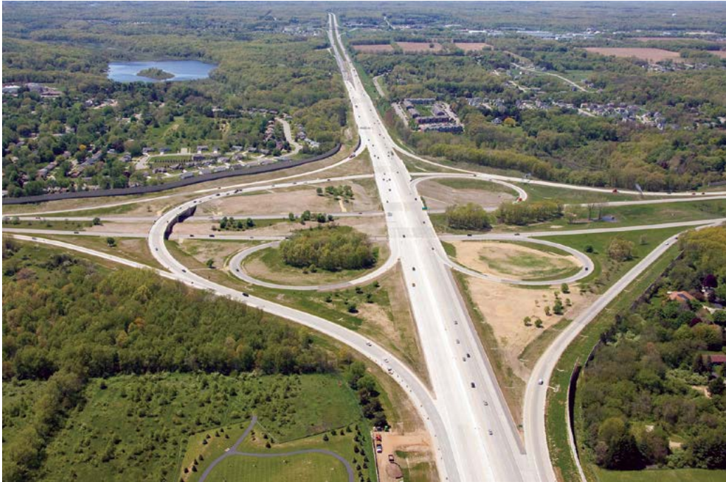
Figure 10-42. Four-Leg Interchange, Cloverleaf with a Semidirect Connection
