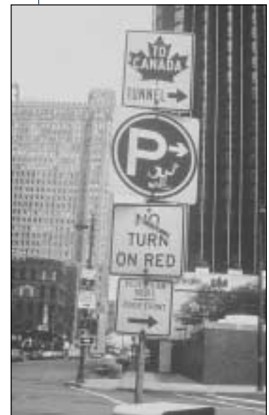
Exhibit 4-10. Poorly located NO TURN ON RED Sign (11).
