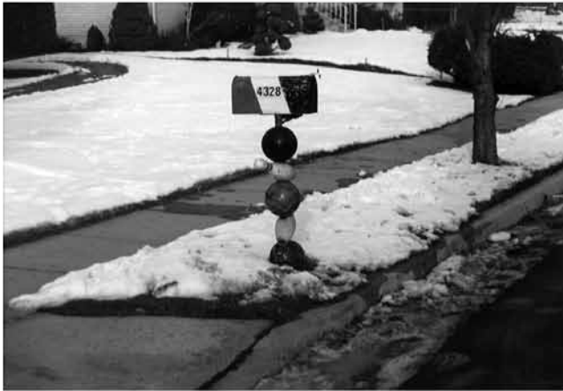
Figure 11-2. Examples of Hazardous Single Mailbox Installations
