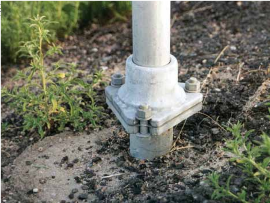
Figure 4-9. Multidirectional Slip Base for Small Signs
