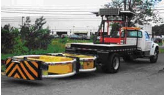
Figure 9-27. TMA with Energy-Absorbing Cartridge
