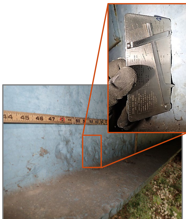
Photo 12 – Cleaned and painting pitting up to 1/4" deep on the bottom 5" of the south web of Beam 7 in Span 3 adjacent to Pier 2, looking northeast.
