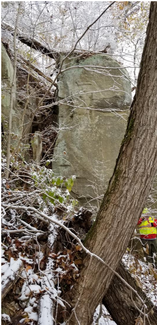
Large jointed block pulling away from slope – 2-foot joint near base, but joint near top is 7-foot wide Total block size is 26' wide x 30' high x 16' deep
