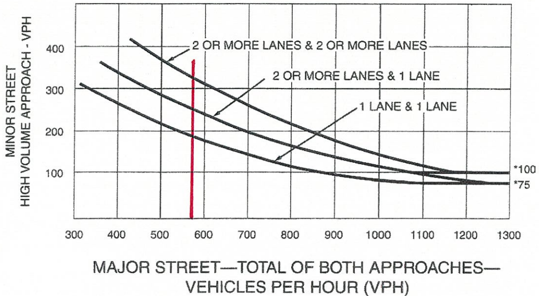
Figure 4C-4. Warrant 3, Peak Hour (70% Factor) (COMMUNITY LESS THAN 10,000 POPULATION OR ABOVE 70 km/h (40 mph) ON MAJOR STREET)
